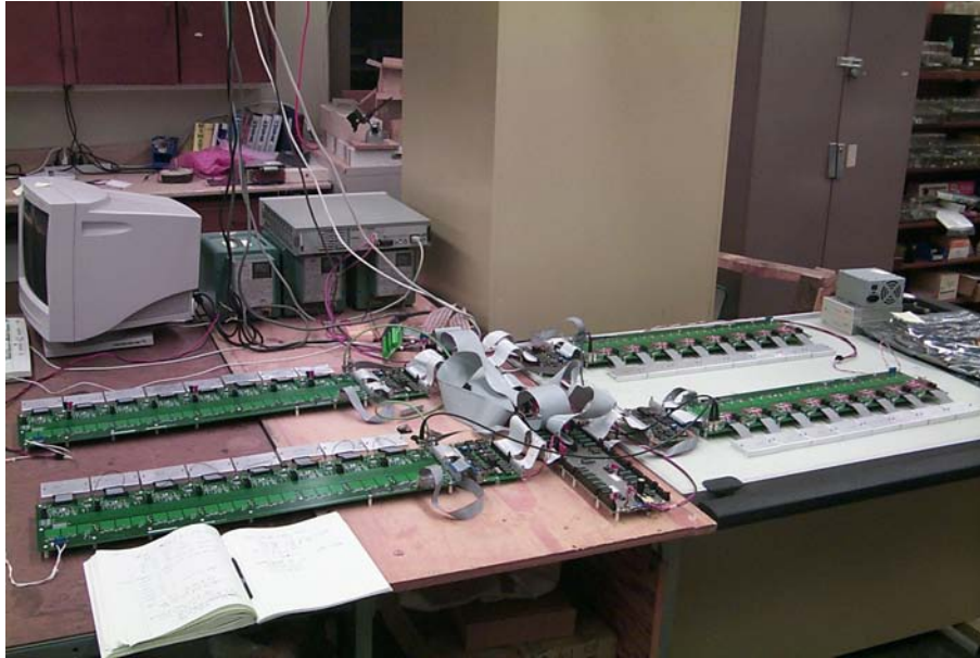
Figure 2: This photograph shows the burn-in stand as used for the close-out portion of the hybrid burn-in project. Here the stand is shown with the maximum capacity of 32 hybrids (the 32 silver rectangles that are lined up in 4 rows).
