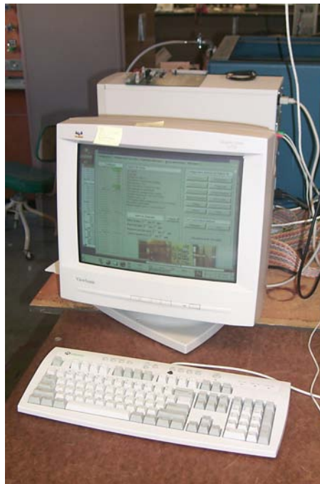
Figure 3: This Linux PC, which is running the Hybrid Monitor burn-in control program (see section 3), contains the three PCI cards discussed in section 2.2.
