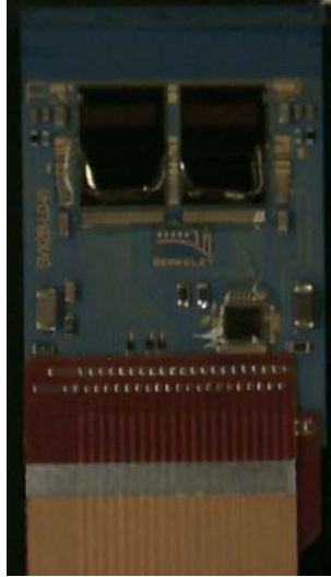
Figure 9: In this picture of a 2-chip hybrid, the two SVX4 chips are visible, along with yellow connectors that lead to a larger adapter board (not shown) that interfaces with the MPX.
