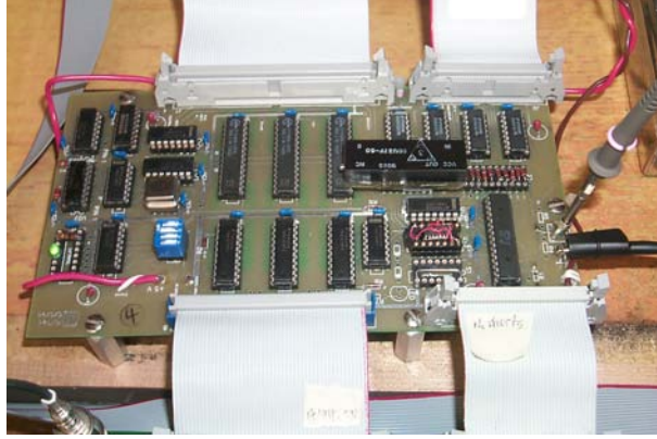
Figure 6: Each pattern board contains a FIFO for sending patterns to the hybrids and a FIFO for receiving data coming from the hybrids. They also contain the oscillator chip that controls the send and receive rates of these FIFOs, and thus is indirectly related to the front-end and back-end clocks of the hybrids. More information about the pattern boards is available in section 2.5.
